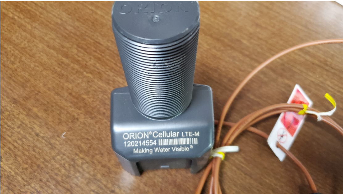
LTE Cellular Transmitter for Advanced Meter Analytics (AMA)
