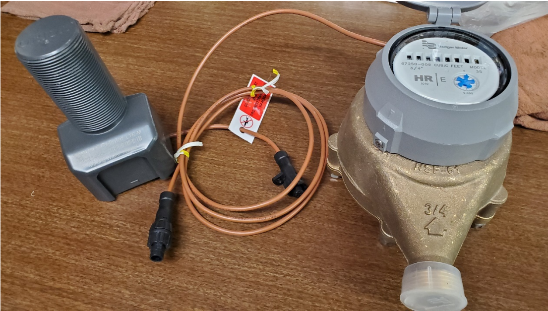
Water Meter and LTE Cellular Transmitter for Automated Meter Reading (AMR) and Leakage Notifications
