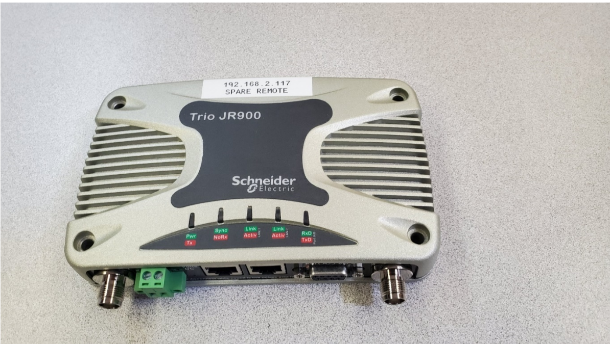
Replacement radios installed at 17 locations
