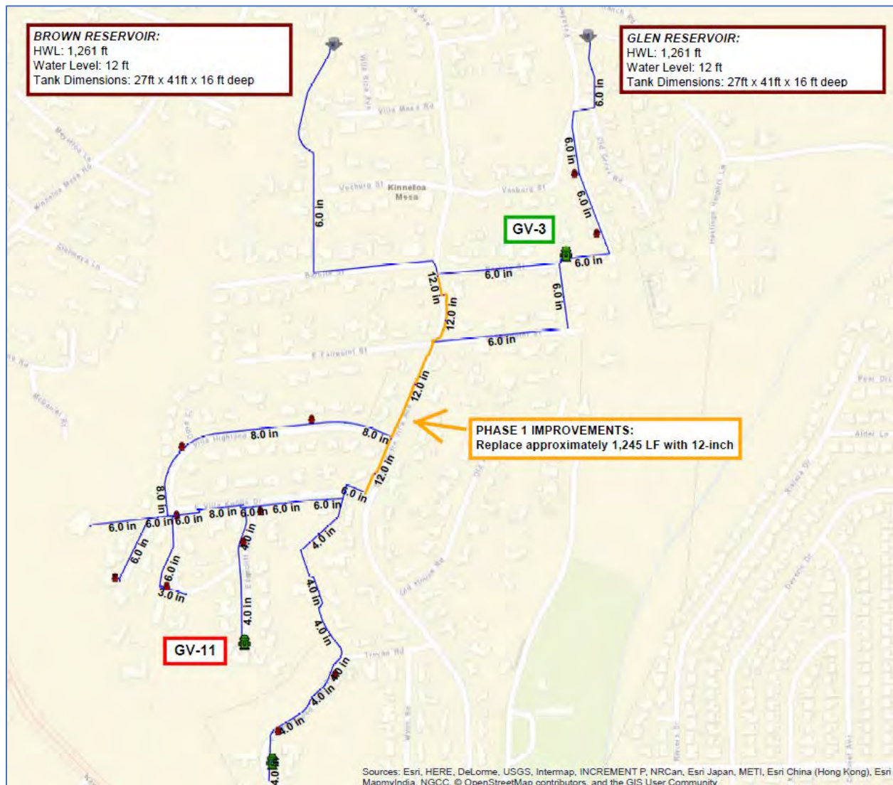
Figure 3 – Phase 1 Improvements Configuration
